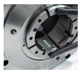
Clamping force or grip force is adjusted by screwing the collet in or out of the chuck. Grip force is increased by the clockwise rotation of the collet. Maximum clamping force is achieved when the indicator pins are flush with the counterbores in the faceplate. To reduce the grip force, rotate the collet counterclockwise until the desired grip is attained. With the force less than maximum, the indicator pins will sit at a position below flush with the counterbores.
