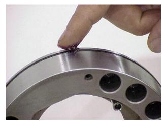
Apply a light coat of grease to both o-rings on the piston and to the I.D. of the body. Gently slide the piston into the chuck body taking care not to wedge the piston in the body.
