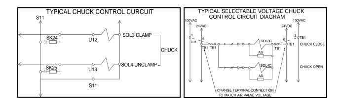
Locate the terminal strip in the electrical cabinet that has the connections for the Chuck Open and Chuck Close solenoids. Locate an area on the electrical cabinet near this terminal strip for the air valves' power cord to enter the cabinet. Drill a pilot hole and use a ½ chassis punch to punch out a hole for the cord grip.
