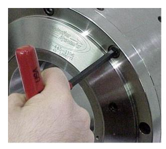
Install the faceplate/pusher combination on the chuck, making sure the indicator pins line up with the holes in the faceplate. Twist the faceplate/pusher combination while on the chuck so the bolt holes in the faceplate line up with the threaded holes in the chuck body.
