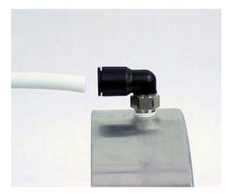
Connect air supply from the valve to the gland housing using the  $\frac{1}{2}$ " airline supplied in the kit. The port in the gland housing is tapped  $\frac{3}{8} - 18$  NPT. Cut off any excess airline and tie up loose or drooping line with wire ties.
