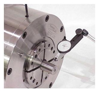
For high precision work, indicate the faceplate in using a piece of ground stock held in the collet pads. This procedure should be performed each time the collet or pads are replaced, if the accuracy requirements justify it.
