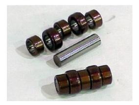
Remove the roller and axle assemblies and set on a clean surface until re-assembly.
