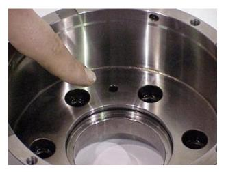
The gland can now be tested for operation and leaks at this point. Turn on the air supply to the valve. Use the foot pedal or chuck open/close switch to open the chuck. Air will blow out the feed holes in the inside of the chuck. There should **NOT** be air leaking from around the body/gland housing interface. With the air off, and the spindle in high gear, the spindle should rotate easily.
