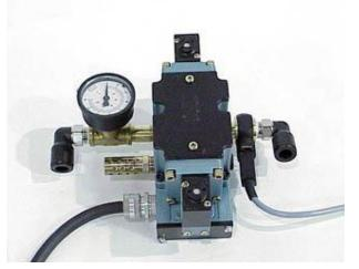
If necessary wire the confirmation switch into the machine according to the electrical diagram supplied with the machine. Look at the manufactures wiring diagram. The chuck control circuits should look something like those shown below. Make sure the control circuit voltage matches the voltage printed on the air valve. Most lathes use 24VDC or 100 VAC to control the chuck solenoid.
