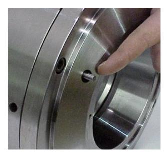
Turn on the air supply to the lathe. The assembled chuck can now be actuated. The pusher will retract when the chuck is opened, or un-chucked, and will move forward when closed, or chucked. Notice the indicator pins moving in and out while the chuck is closed and opened, respectively.
