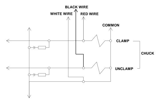
Connect the **WHITE** wire to the **COMMON** side of the solenoids Connect the **BLACK** wire to the **OPEN** signal Connect the **RED** wire to the **CLOSE** signal Connect the **GREEN** wire to **EARTH** Ground
