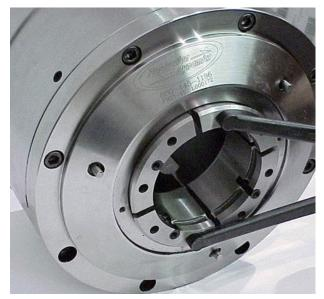
The chuck may release the workpiece due to low grip force. With the pins above flush, the collet grip force drops significantly. Remember, when the pins are extended out all the way, the collet is open and the workpiece is released.
