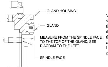
While putting on the Gland Housing be sure to measure for clearance between the chuck and Gland Housing. This distance should be .030" to .040" less than the length from the back of the chuck to where the gland seals. See Illustration below. This will allow clearance for the chuck to rotate freely.
