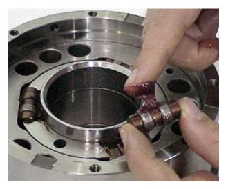
Install the roller and axle assemblies into the ramp. **LIGHTLY** grease the assembly to hold them in place for installation, and for lubrication after assembly.
